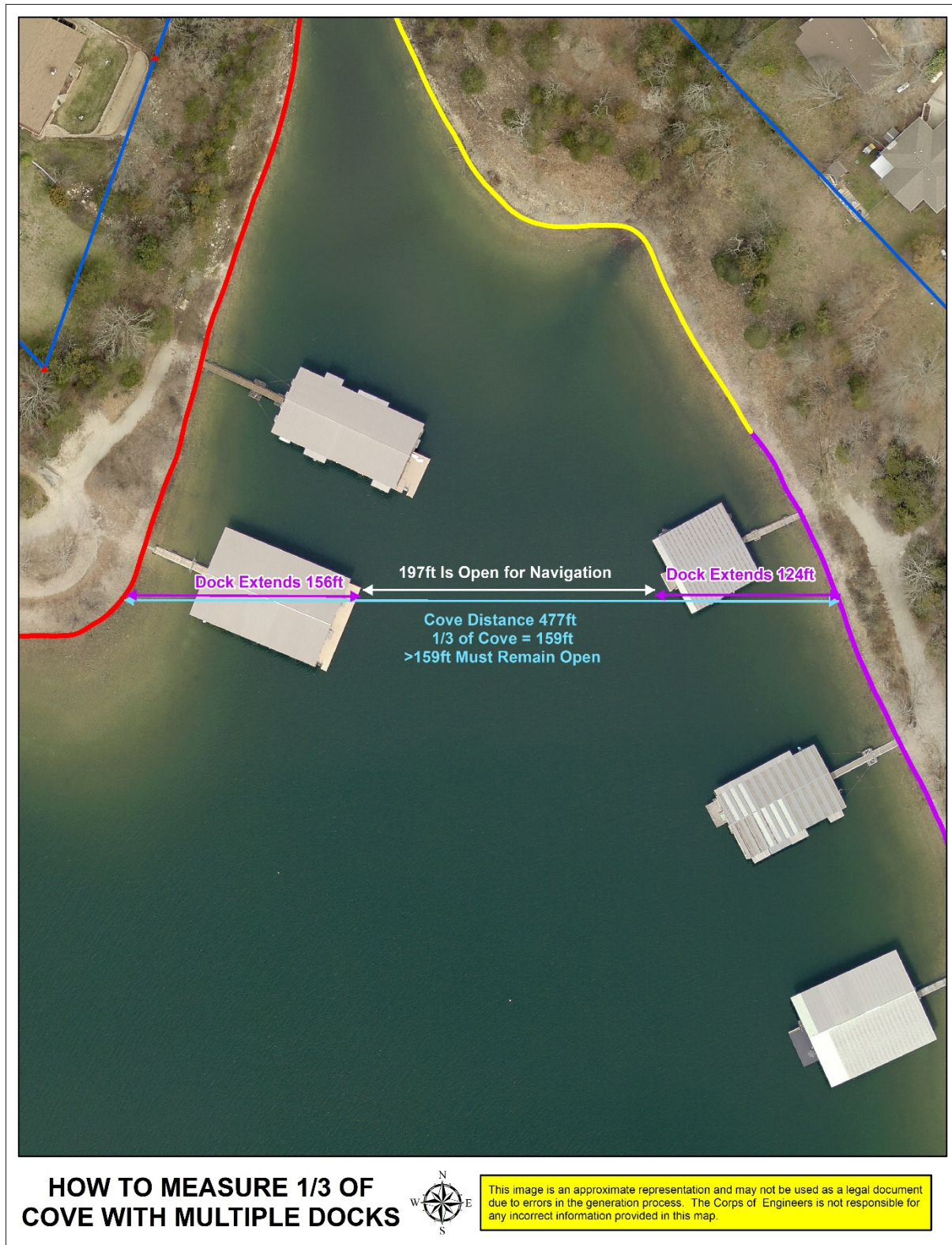
FIGURE 3: HOW TO MEASURE 1/3 COVE WITH MULTIPLE DOCKS
