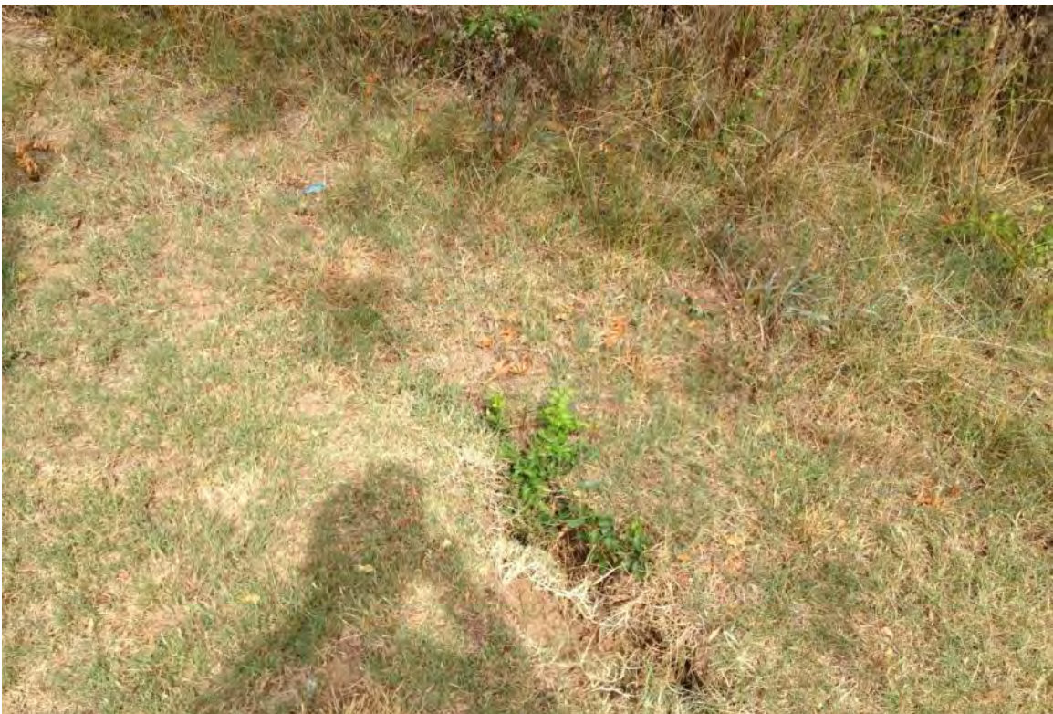
Photo 15 Area 3: Tension cracks are visible (center of frame) along a length of the eroding streambank on Town Branch. The cracks are located approximately 10 feet from the edge of the streambank.
