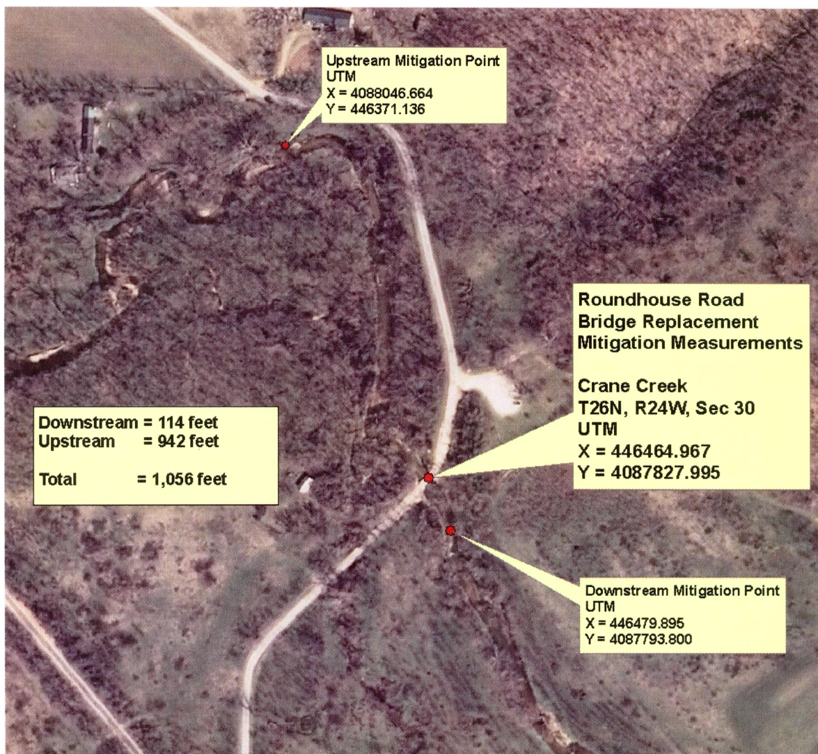
Figure 2. Aerial Map of Roundhouse Road bridge replacement site with mitigation measurements and UTM coordinates listed.
