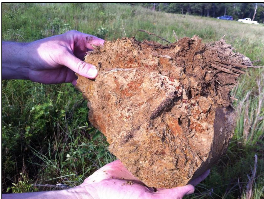
Photo 6: Wetland soil sampling showing iron oxidation lenses
