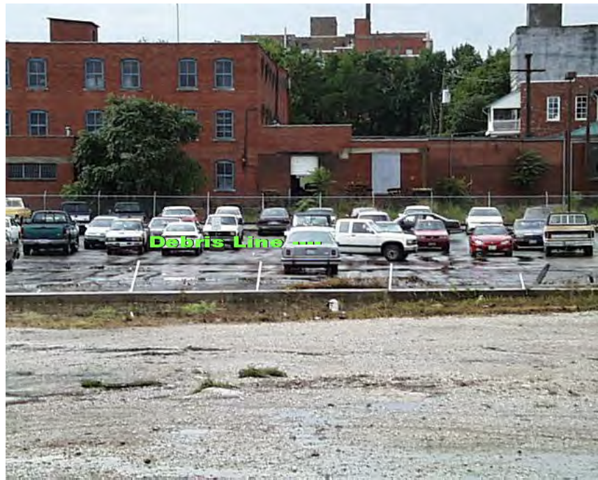
Lower Branch of Jordan Creek, at 410 N Boonville Avenue (between Lower Branch RS 14607 & 14941). The ground elevation is estimated at 1269.5 with an estimated distance of 3.5-ft to the top of the trunk. This photo was taken after flood waters receded on July 12, 2000. See Appendix F for WSE comparison.
