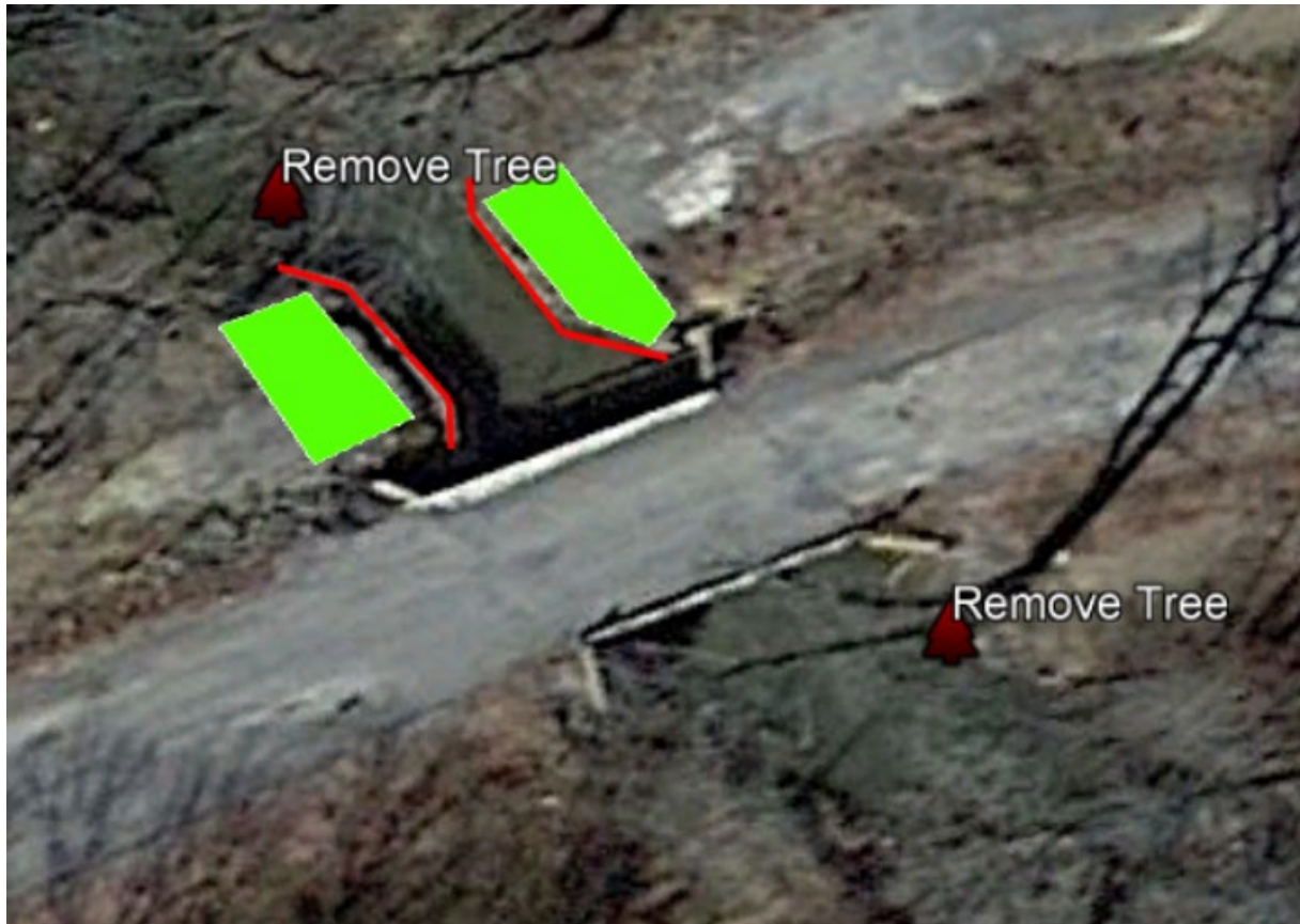
Figure 18. Mortar Creek Recommended Plan. Green areas show general area of streambank protection, red lines represent the old bridge abutments to be removed and the dark red figures show the tree removals. Not shown: riprap placement around all four wingwalls.
