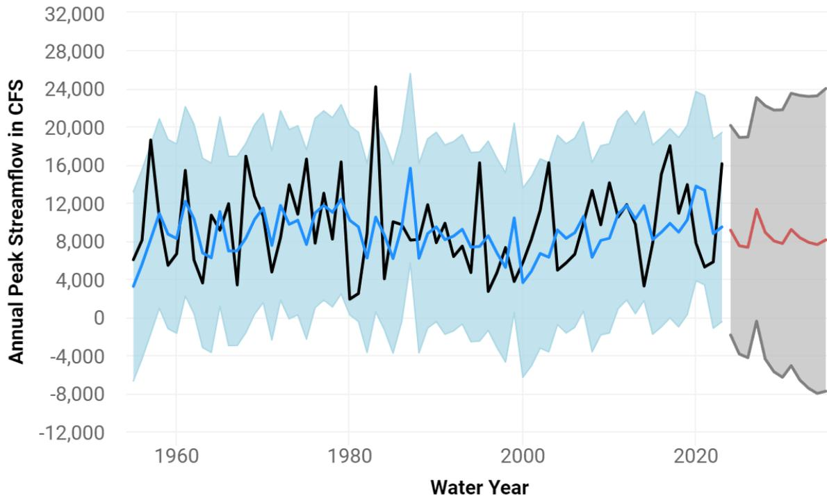
**Figure 20. Auto Regressive Integrated Moving Average (ARIMA) Model Forecast for Cadron Creek near Guy, AR**
