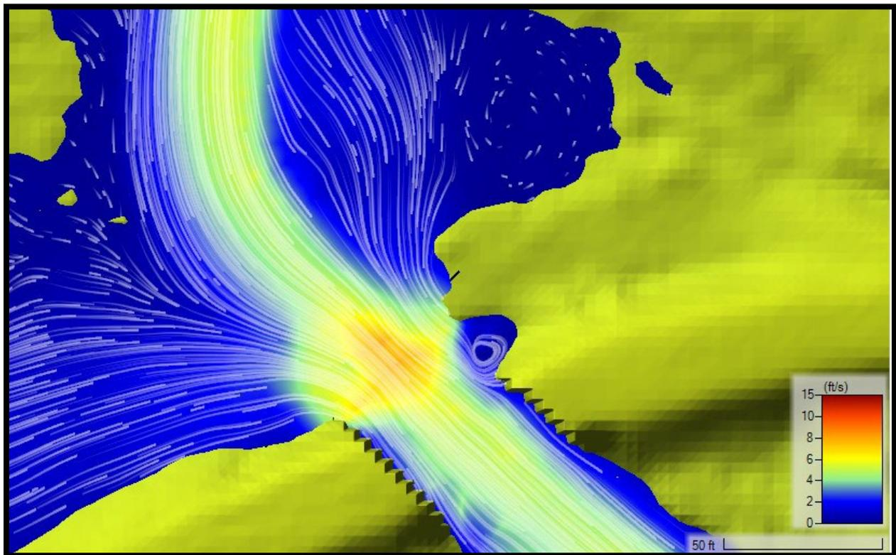
**Figure 5. Screenshot from 2D RAS Model with Particle Tracers and Velocity Map for 50% AEP Flow**
