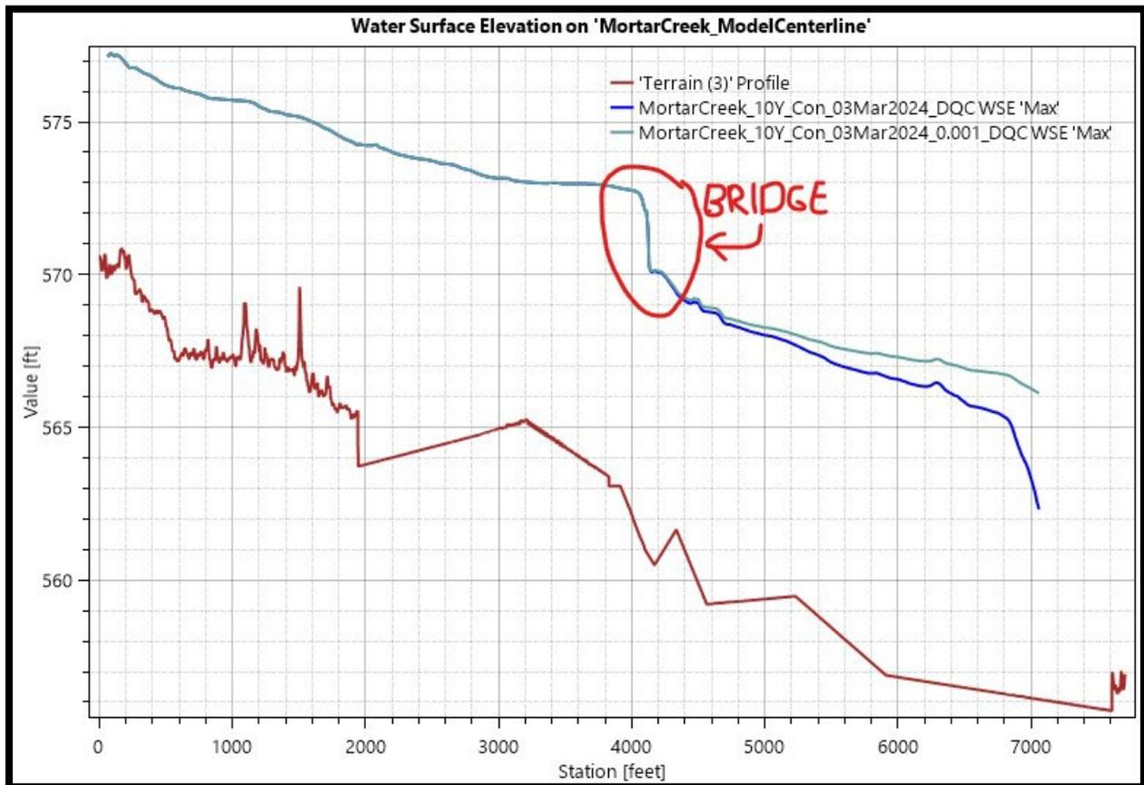
Figure 4. Downstream Boundary Condition Sensitivity
