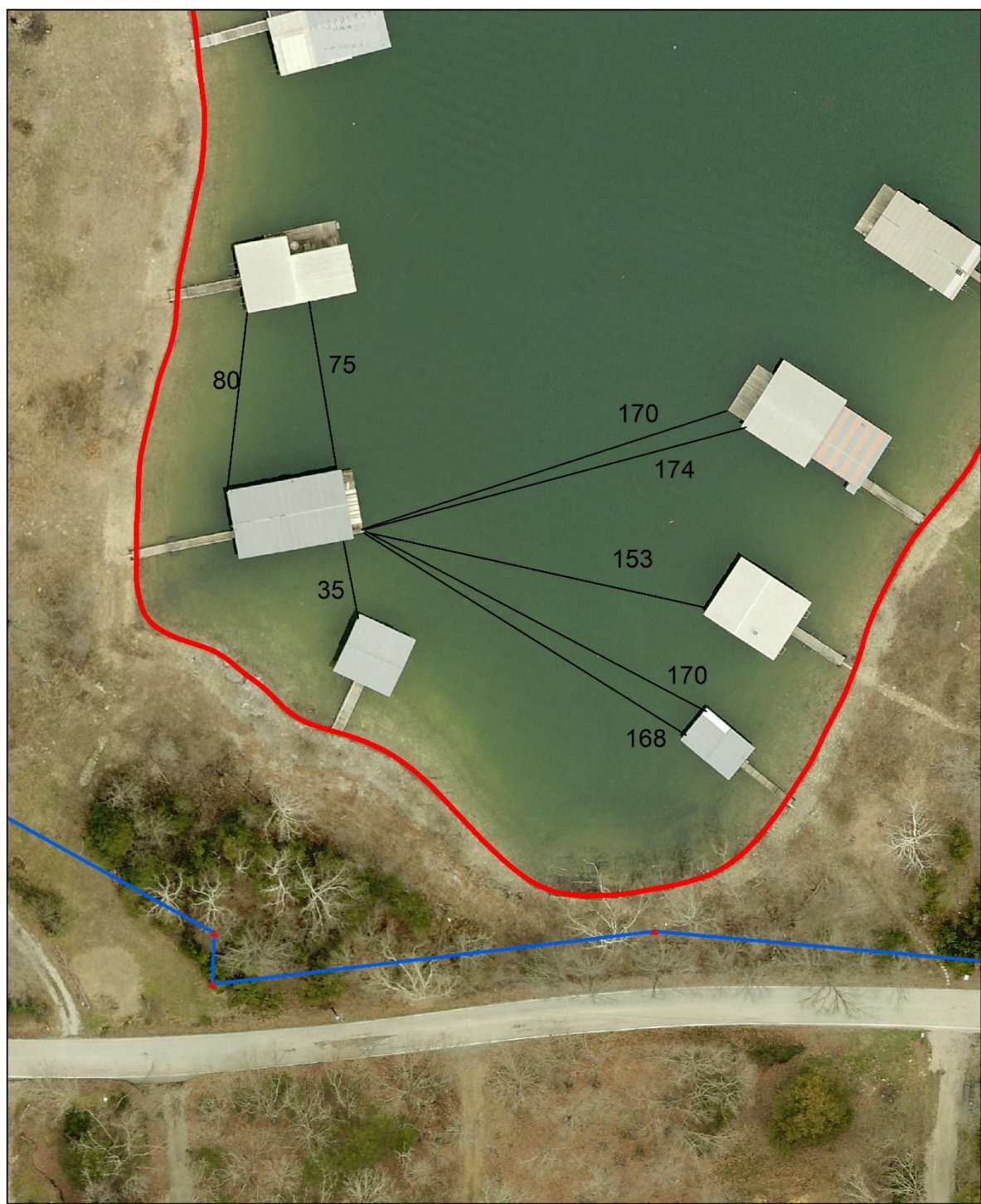
FIGURE 4: HOW TO MEASURE 100' BETWEEN DOCKS
