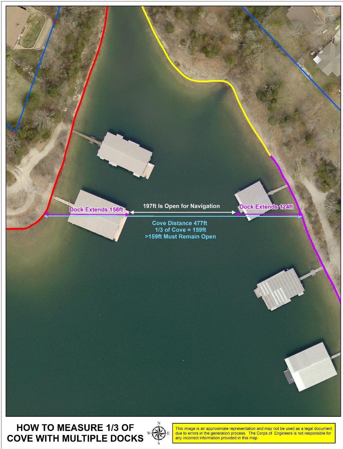
FIGURE 3: HOW TO MEASURE 1/3 COVE WITH MULTIPLE DOCKS
